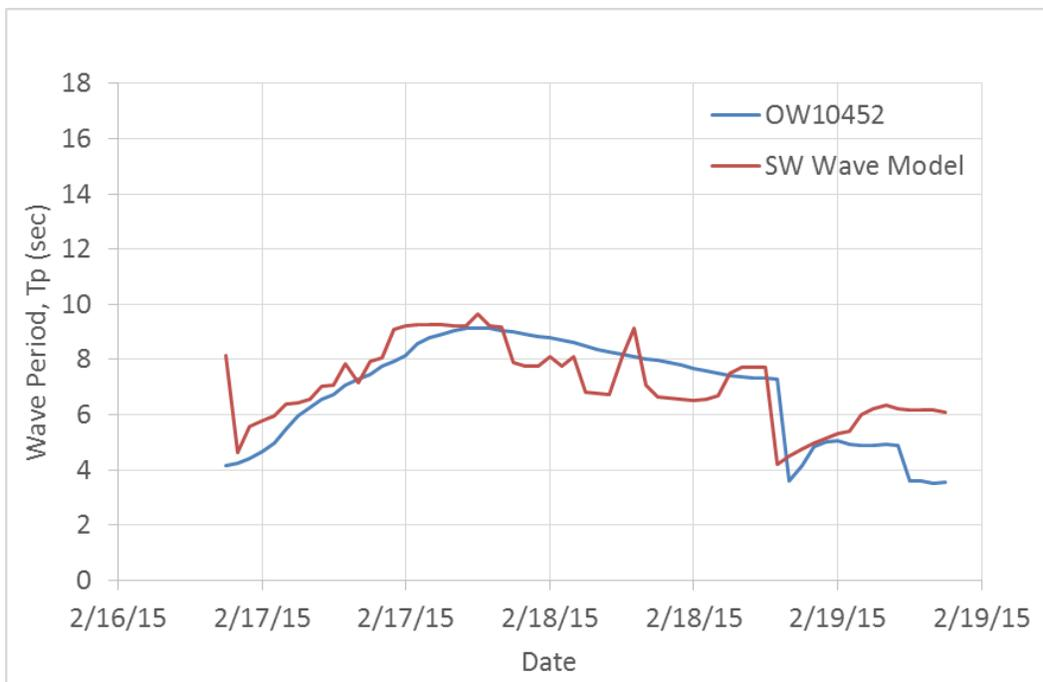
Figure 3-4: Calculated Wave Periods Compared to OW10452 Wave Periods (Open Boundary Conditions: NDBC 41004 Buoy Data)
