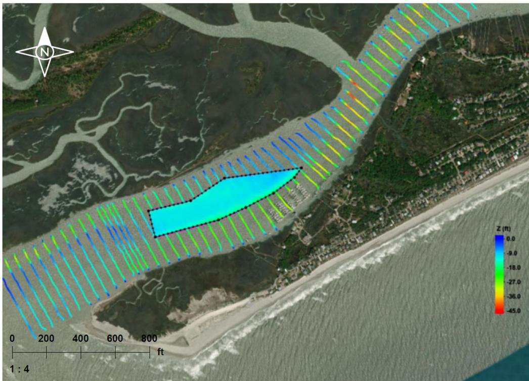
Figure 1: May 2014 bathymetric survey data with interpolated bottom surface TIN overlay.
