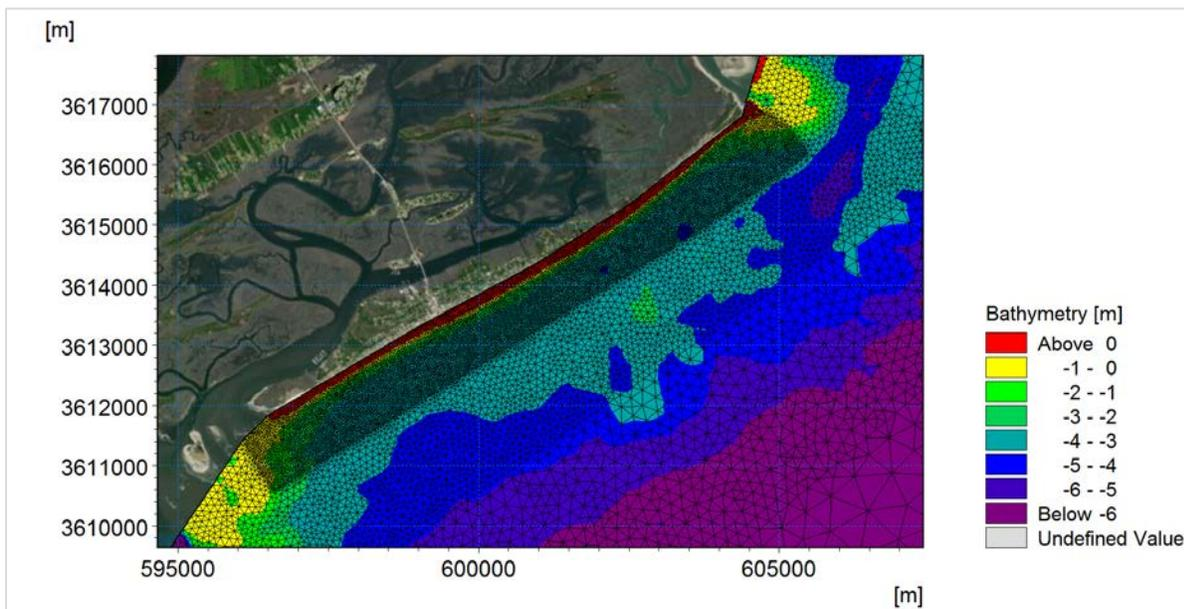
Figure 3-2: Spectral Wave Model Mesh (Project Site)
