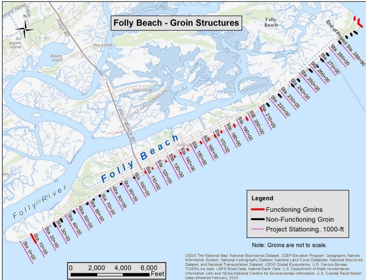
Figure 2-2. Existing Groin Structure Location
