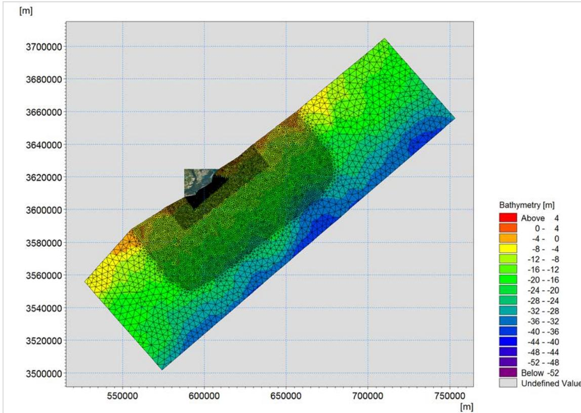
Figure 3-1: Spectral Wave Model Mesh (Entire Area)
