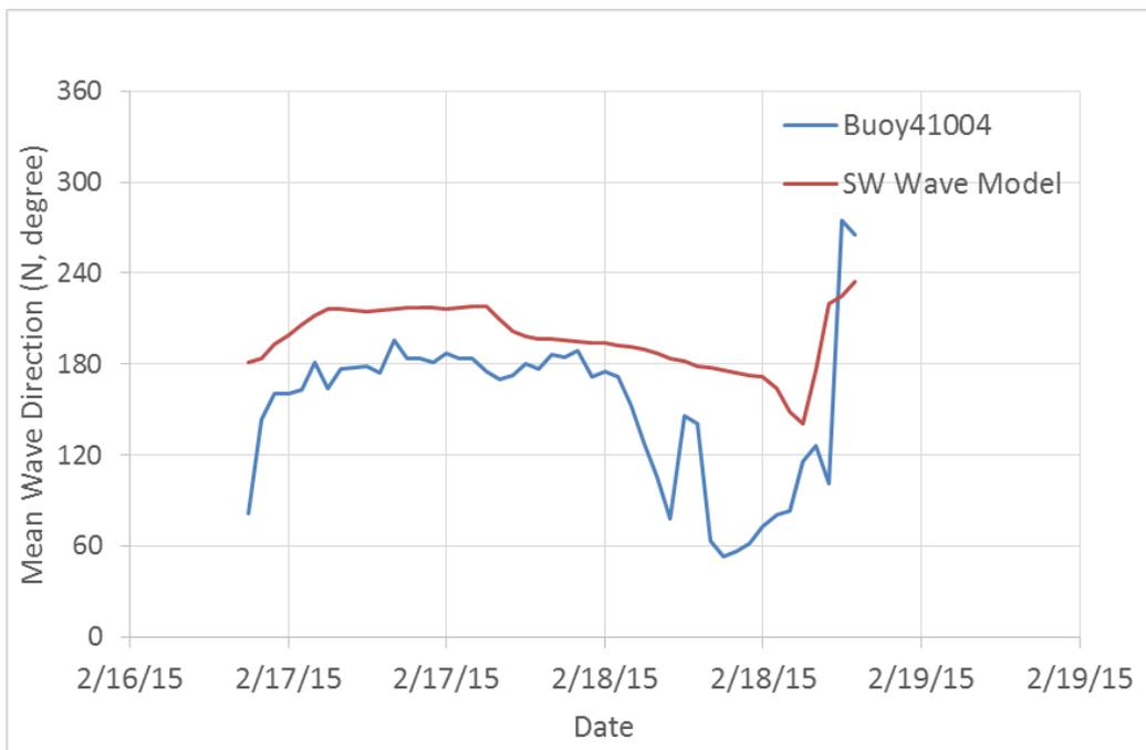
Figure 3-17: Calculated Wave Directions Compared to Buoy41004 Wave Directions (Open Boundary Conditions: NDBC 41004 Buoy Data)
