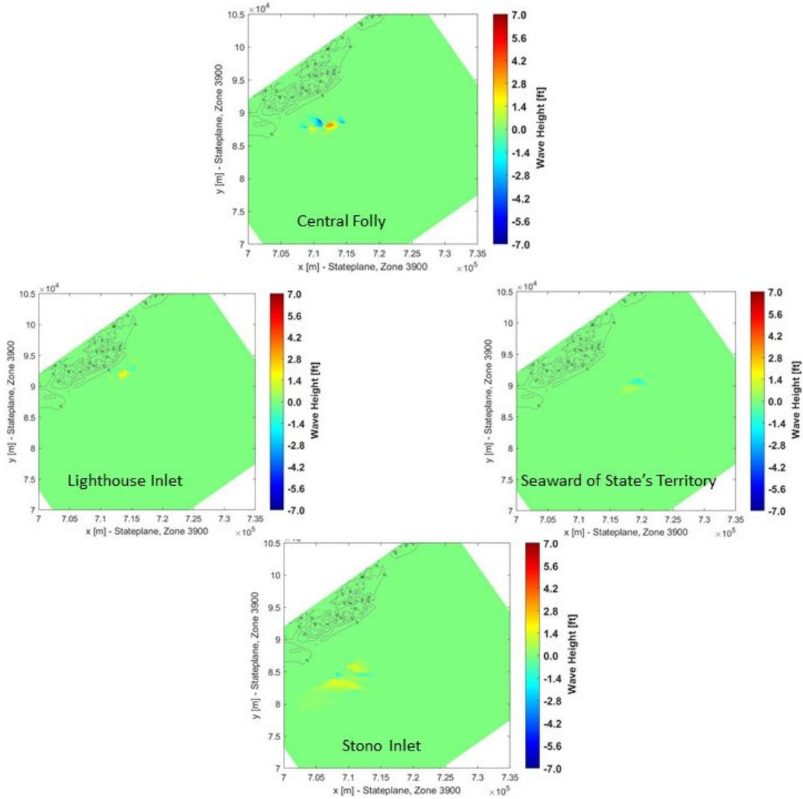
**Figure 5:** Extreme Event Condition at all four borrow areas. Warm tones indicate increases in wave height when compared to the no borrow are simulations and cool tones represent decreases in wave height.
