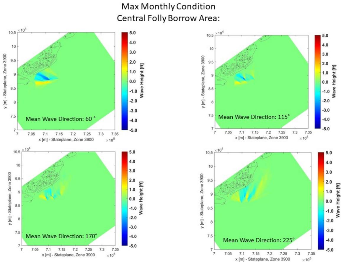
**Figure 4:** Max Monthly Condition at the Central borrow area site. Warm tones indicate increases in wave height when compared to the no borrow are simulations and cool tones represent decreases in wave height.
