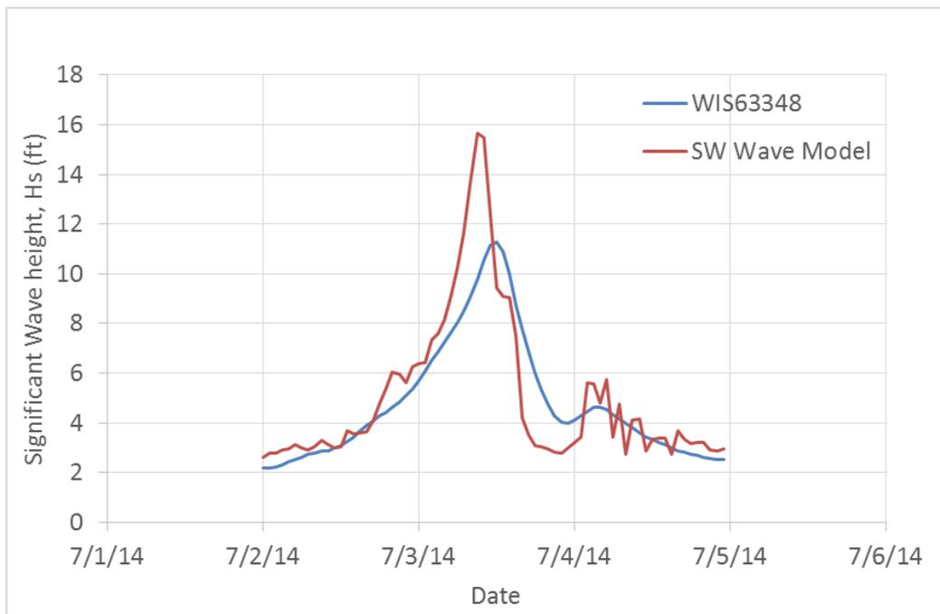
Figure 3-9: Calculated Wave Heights Compared to WIS63348 Wave Heights (Open Boundary Conditions: NDBC 41004 Buoy Data)
