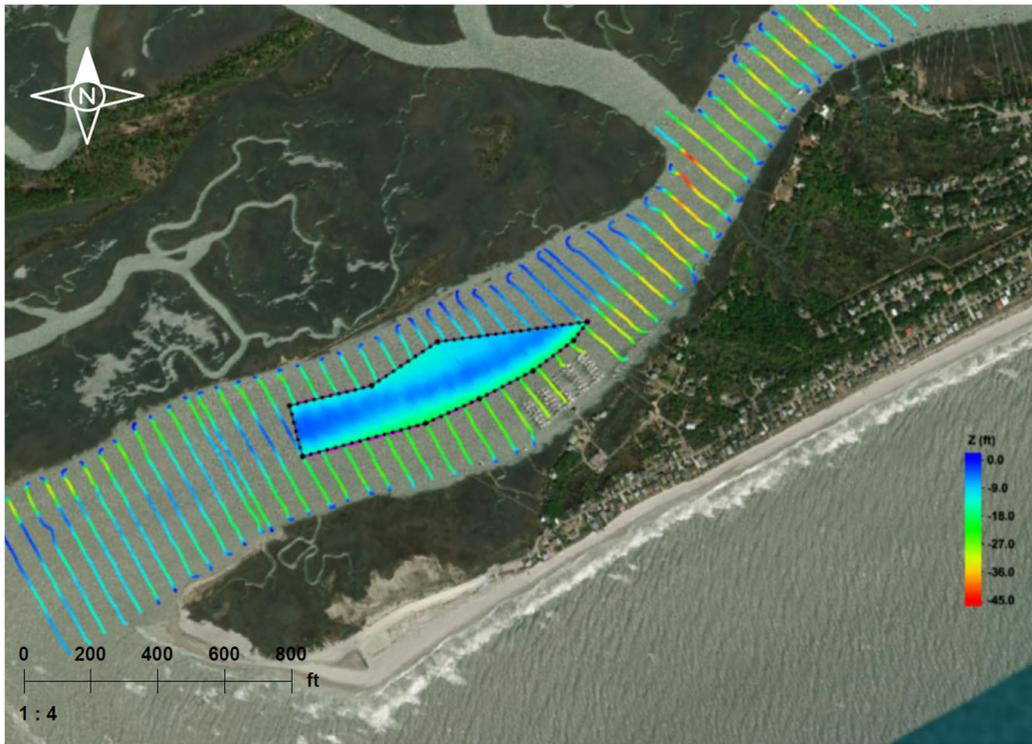
Figure 2: May 2015 bathymetric survey data with interpolated bottom surface TIN overlay.
