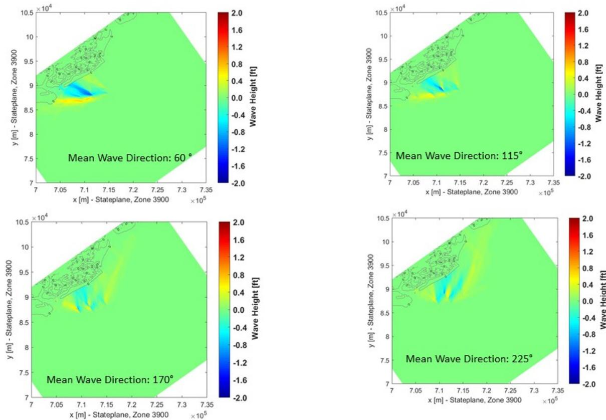
**Figure 3:** Mean monthly condition at the Central borrow area. Warm tones indicate increases in wave height when compared to the no borrow are simulations and cool tones represent decreases in wave height.
