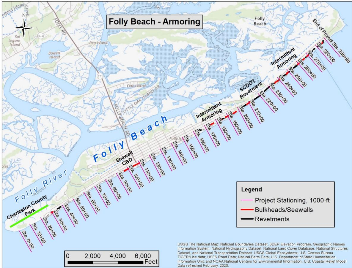
Figure 2-3. Existing Bulkhead, Seawalls and Revetment Sections
