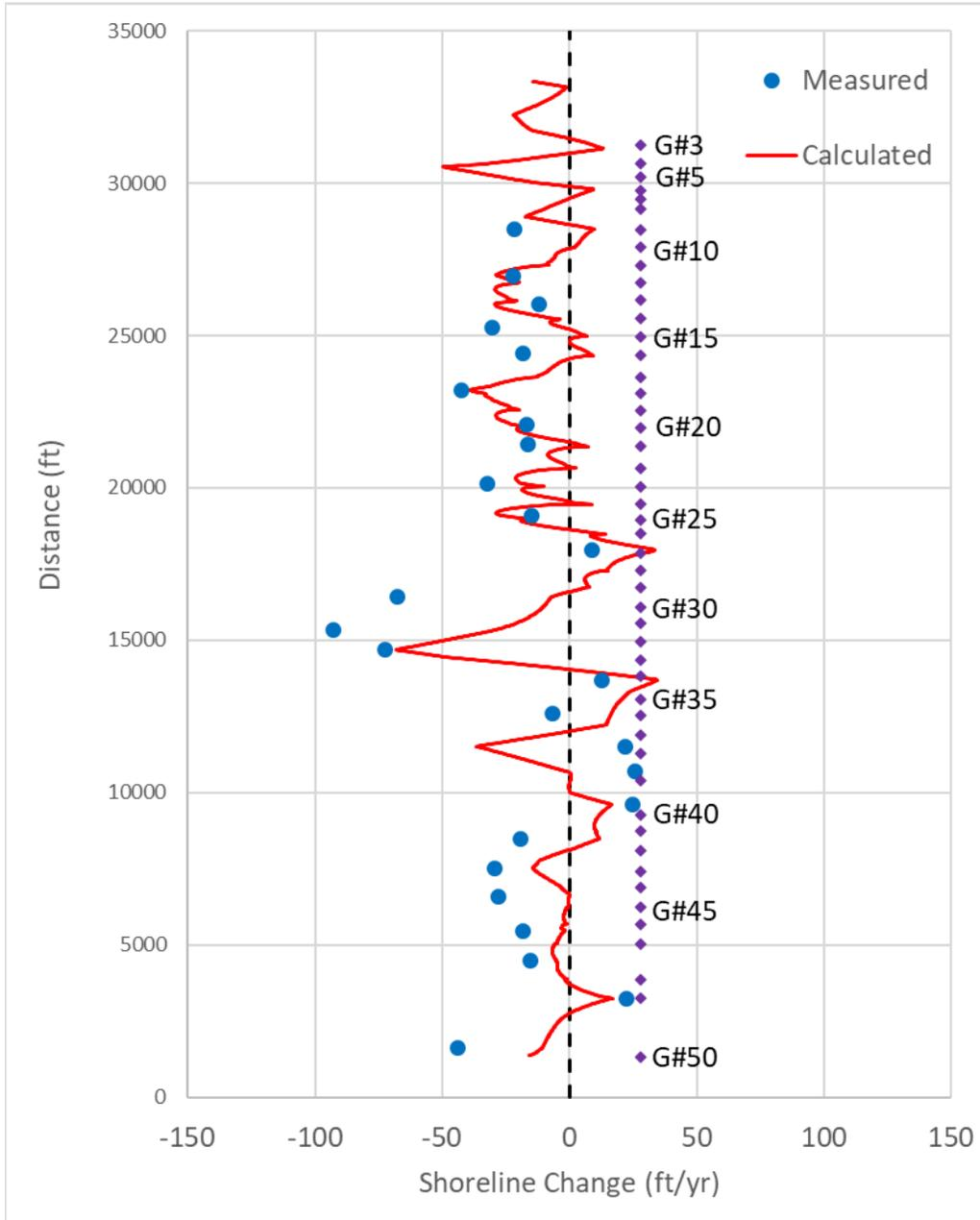
Figure 4-2: Shoreline Model Calibration (Dec. 2016 to Dec. 2017)
